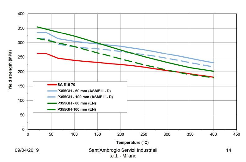
Nominal Design Stresses for Carbon Steel materials SA 516 70 and P355GH (according to EN 10028.2 and to ASME VIII - Creep values based on a lifetime of 100000 hours)
